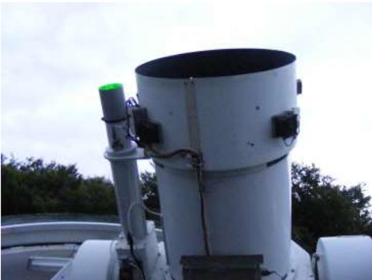
The laser being fired from the refracting telescope on the left, whilst the larger Cassegrain telescope receives the return laser photons
