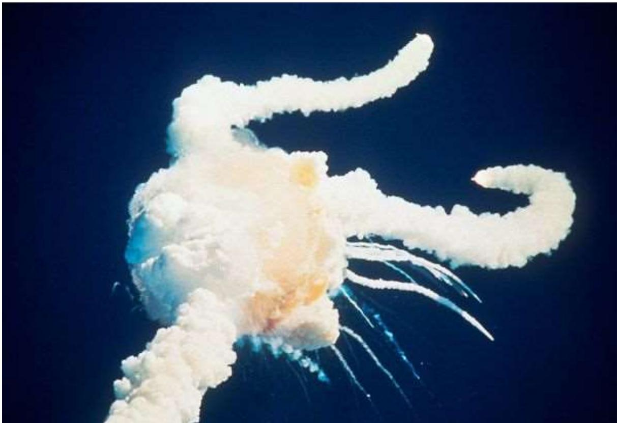
Igniting of the escaping liquid hydrogen and liquid oxygen fuels resulted in a fire ball. The two solid fuel boosters careered off, uncontrolled
