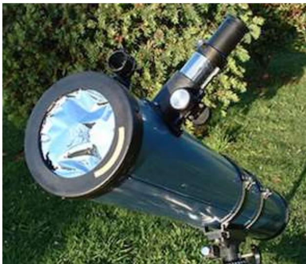
Using a Baader Solar Filter
