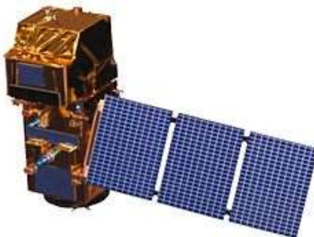
European Space Agency's ESA Sentinel satellites are an earth monitoring system that uses two satellites, 2a and 2b launched 23 June 2015 and 7<sup>th</sup> March 21017 respectively. They are designed for land and sea monitoring, natural disaster mapping and sea ice observations. They circle the Earth 14.3 times a day at a height of 488 miles.
