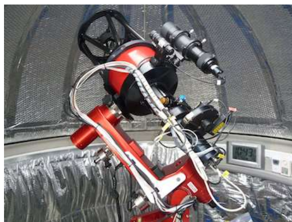
The mount with an IKHAROS 8-inch Ritchey Chretien telescope and a narrow band filter
