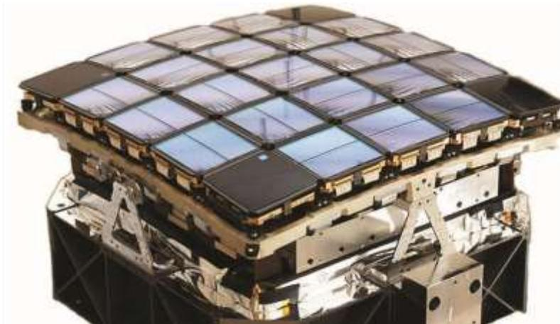
Each one of those silver squares contains 2 CCDs with a resolution of 2,200 x 1,024 pixels. There are 42 of them producing 95 megapixels of data. Each star is allocated a postage stamp of 30 pixels. The star data is read from these pixels every 6 seconds and integrated for 30 minutes before being stored for a monthly transmission to Earth. The monthly download is about 12 gigabytes of data.
