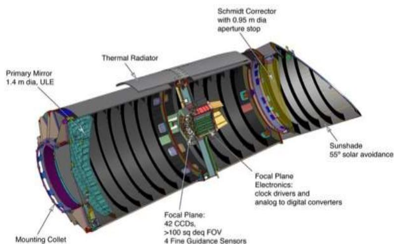
This NASA diagram is of the inside of the Kepler space telescope. It is the fine guidance sensors and the motors that have caused all the problems. The telescope is a Schmidt with a 0.95 metre (37-inch) front corrector plate feeding onto a 1.4 metre primary mirror. The spacecraft weighs 1,039 Kg. The 42 CCDs produce a total of 95 megapixels.
