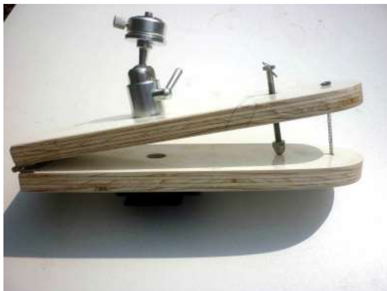
One version of the barn-door tracking device
