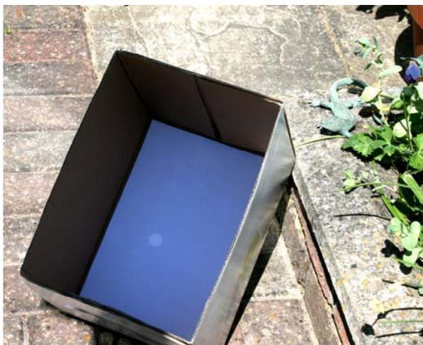
Above is a photograph that I took to demonstrate the principle of pinhole projection. I used an empty A4 paper box with a sheet of white paper in the bottom and made a 3mm hole in the lid. I am holding the lid just over two metres away and keeping it in such a position that the box is completely in its shadow. This makes the image easier to see although it is quite small.
